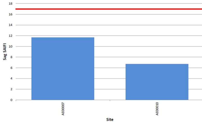
Figure 3-8: Voltage sag performance – 6.6 kV site
